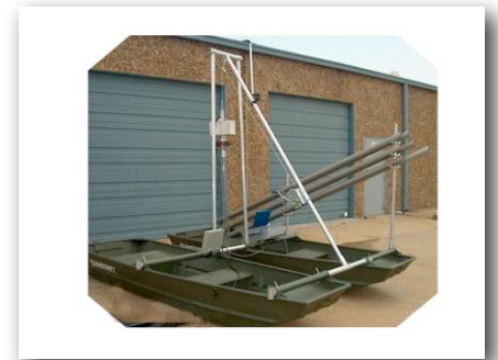
DJB-1243 Setup with Vibe-Core and Core Tube on Rack
